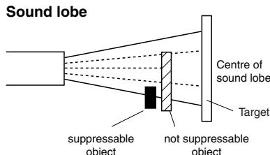
The suppression of the disturbing target is effected through reduction of the response sensitivity. This figure shows its effect on the response characteristics of the sensor. The sensor is preset on step 1 by the manufacturer.
